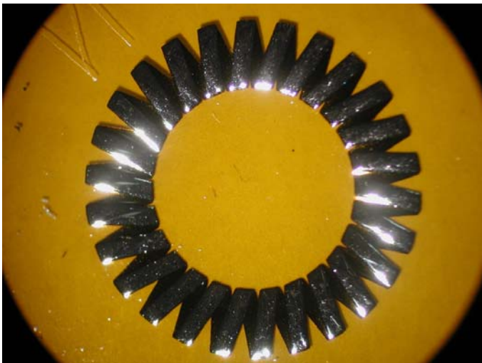
Fig. 10. Photomicrograph of N and P Si/SiGe Quantum Well Module During Fabrication with a Stainless Steel Mask: N-type Deposited on One Side of Kapton™ and P-type on the Opposite Side
