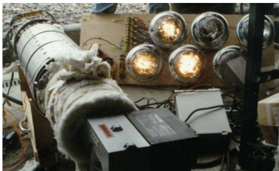
Figure 5. Hot air blower TEG test setup with car light bulbs load
