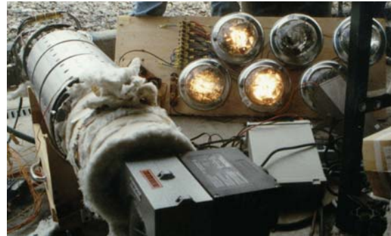
Figure 10 —Hot air blower TEG test setup with car light bulbs load.
