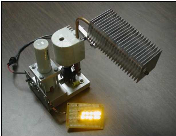
Figure 1: Milliwatt Butane-Heated Generator
