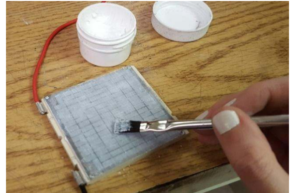
Figure 4: Spreading Thermal Grease
